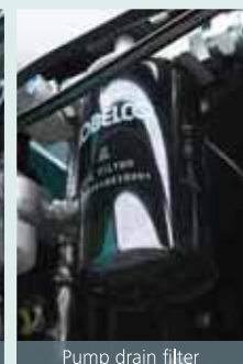
Pump drain filter
