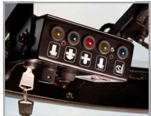
Twistlock module with indicator lights
